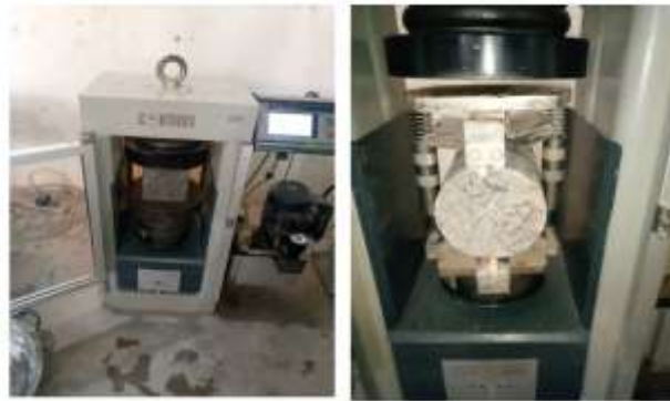
Figure 1. compression and Split Tensile test set-up
