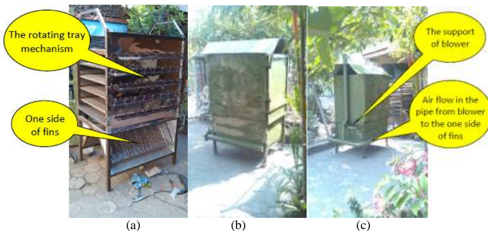
Figure 3. (a) Cocoa beans dryer in manufacture processing, (b) The side view, and (c) The behindview of Cocoa beans dryer.
