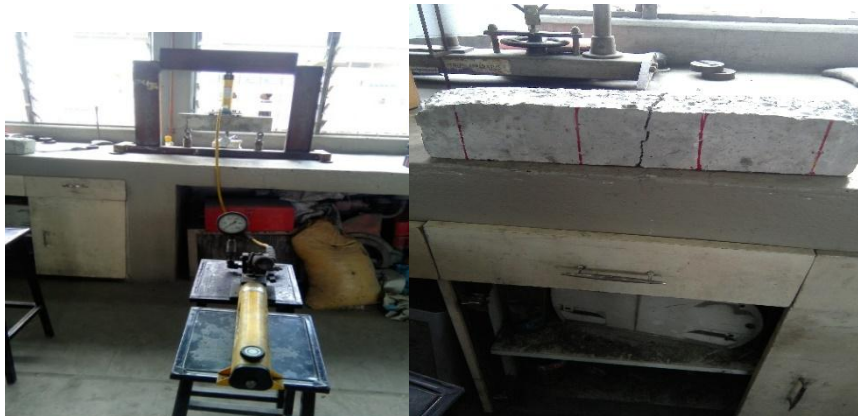
Plate 3 Progress photographs of Split Tensile and Flexural Strength Test
