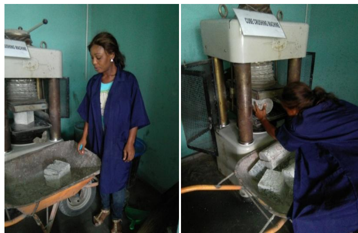
Plate 2. Progress Photograph for Cube Compression Test
