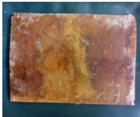
Fig. 5. Manufactured rattan fiber laminate.
