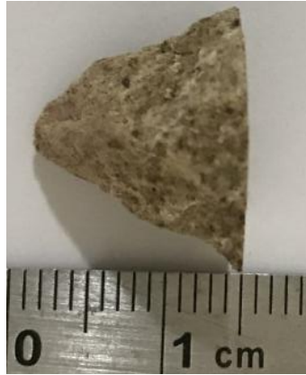
Fig.7. Sintered fracture that had the best apparent mechanical performance, containing 30% glass embedded with 37.5 \mu\text{m} particle diameter, sintered at 1100°C
