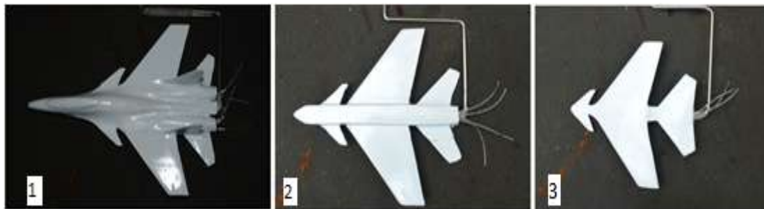
Fig.2. Finishing of BBTF model, 1) The original fuselage, 2) symmetric wall fuselage, and 3) without fuselage
