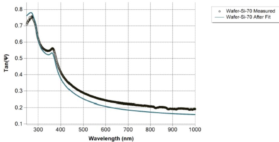
Figure 3: Relationship between experimental and theoretical  $\psi$  tangent.
