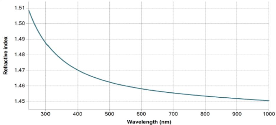
Figure 5: Refractive index for layer vs. Wavelength.
