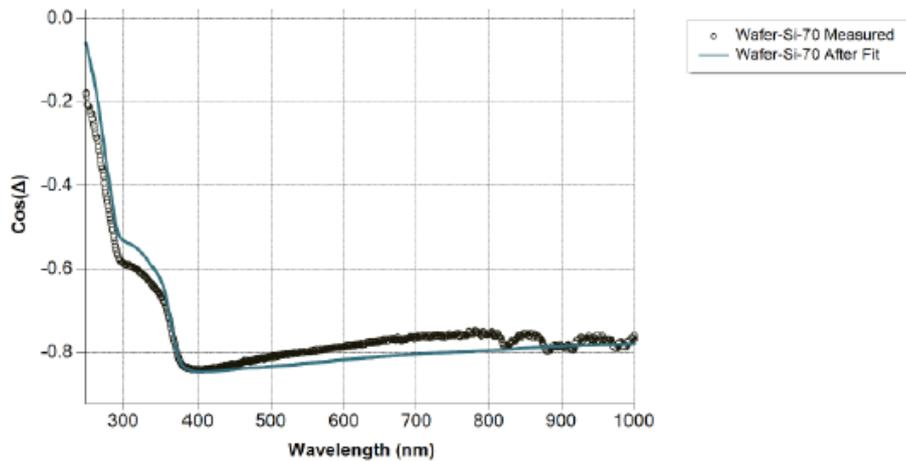
Figure 4: Relationship between experimental and theoretical  $\Delta$  cosine.
