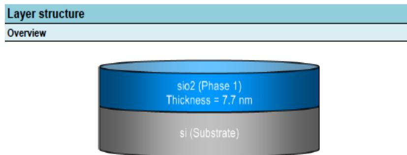
**Figure 1: Overview of the structure of the semiconductor sample.**
