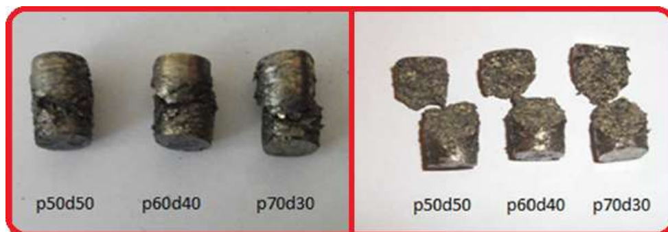
Figure 7. The fracture surfaces of the produced composite materials
