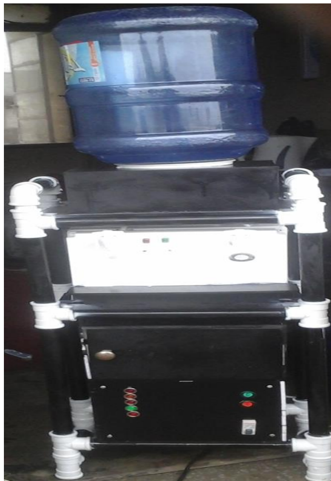
Figure 6: Pictorial view of fabricated Hot and Cold Water Dispenser with Inbuilt inverter
