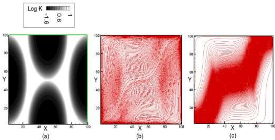
Figure.9. a quarter five spot model with a 100×100 grid-blocks, (a)Permeability field for problem 2; (b) and (c) show the streamlines traced by the MSM (249 SL) and SSM (380 SL).
