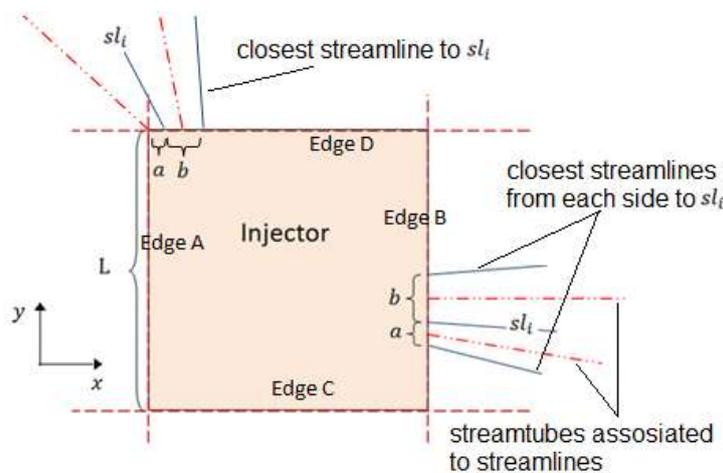
Figure.4. a schematic representation of the streamlines and 2D streamtubes considered around them to determine the associated flux for each streamline.
