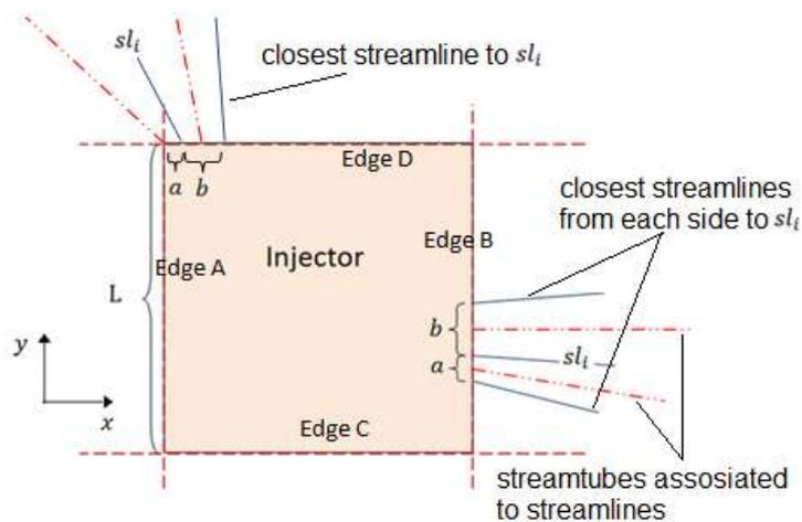
Figure.4. a schematic representation of the streamlines and 2D streamtubes considered around them to determine the associated flux for each streamline.
