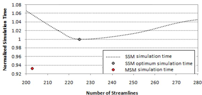
Figure.8.shows the Normalized Simulation time for SSM with different number of streamlines (224 streamlines in optimum point) and MSM with 203 streamlines for a heterogeneous quarter five spot problem 1.
