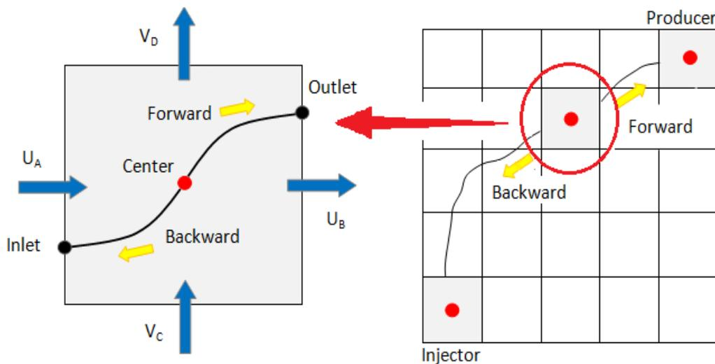
Figure.1. (a) Tracing streamline forward and backward from the center of the grid-block to its faces, and (b) from grid-block faces to injector and producer using Pollack's method.
