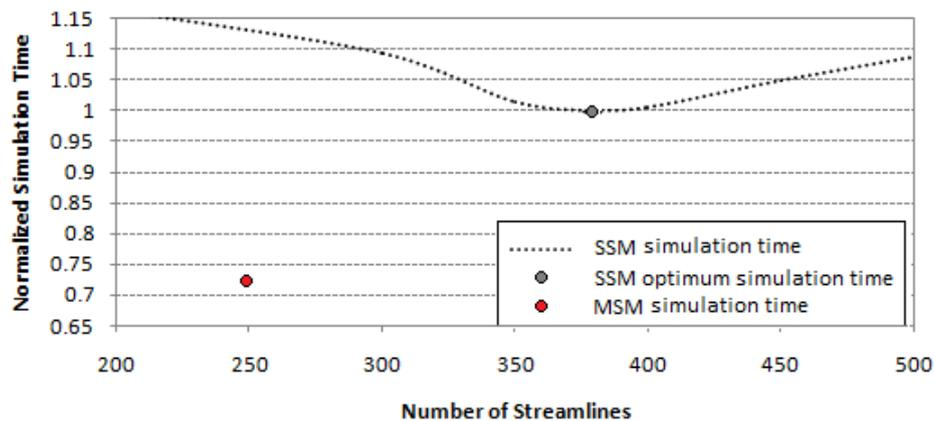
Figure.10.shows the Normalized Simulation time for SSM with different number of streamlines (380 streamlines in optimum point) and MSM with 249 streamlines for a heterogeneous quarter five spot problem 2.
