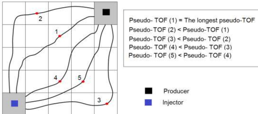
Figure.2. the sequence over which streamlines are traced using MSM; the pseudo-TOF for grid-blocks defined by the magnitude of the velocity gradient is the parameter upon which the tracing is performed until all grid-blocks contain at least one streamlines.
