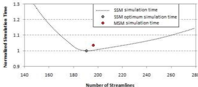
Figure.6. shows the Normalized Simulation time for SSM with different number of streamlines (190 streamlines in optimum point) and MSM with 196 streamlines for a homogeneous quarter five spot model.
