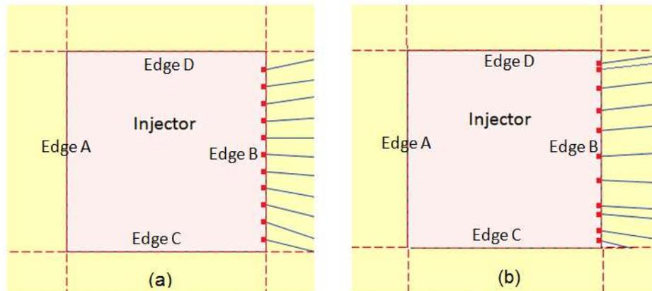
Figure.3. Streamline and injector face connection in (a) SSM and (b) MSM. Squares show a place where streamlines connect to the face of the injector grid. This connection is uniform in SSM, while non-uniform for the MSM.
