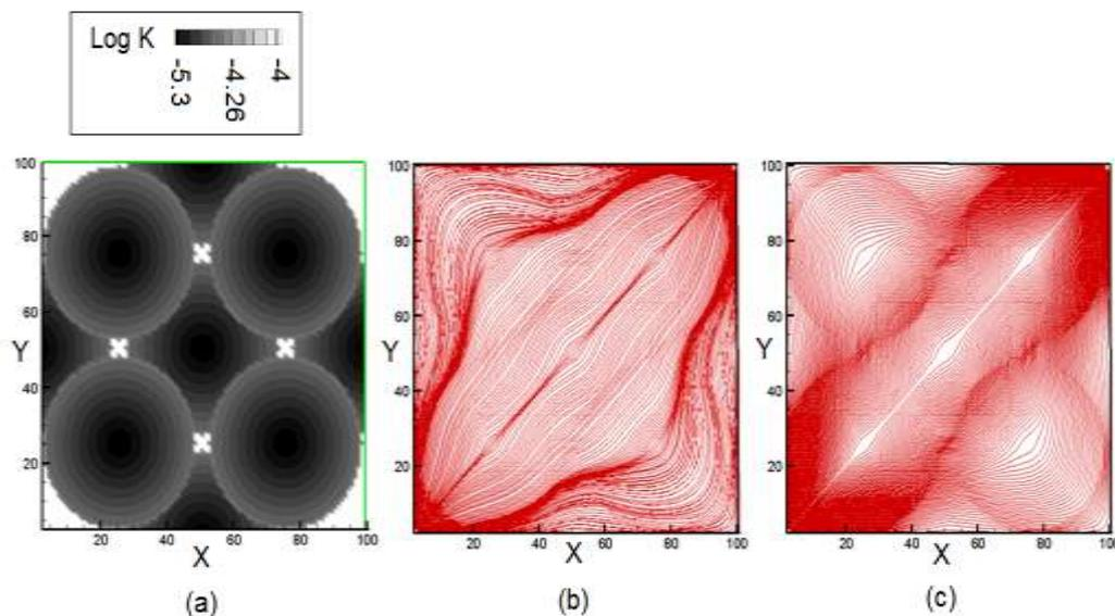
Figure.7. A heterogeneous ( $100 \times 100$ ) problem 1; Panel (a) shows the permeability field and panel (b) and (c) show the streamlines traced by the MSM (203 SL) and SSM (224 SL).
