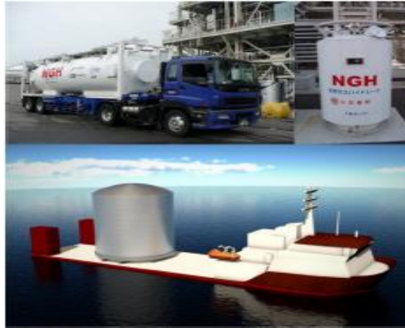
Figure 3: Three-dimensional illustration of Hydrates transportation (Raine et al, 2015 and Takaoki, 2006)
