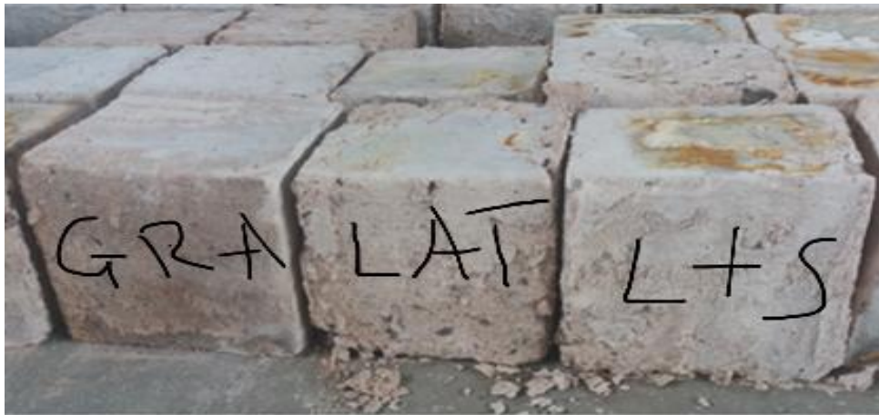
Fig. 4: Deterioration for M25 concrete at 90 days
