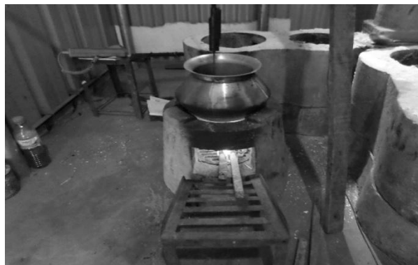
Fig. 13: Single mouth concrete cook stove during operation.
