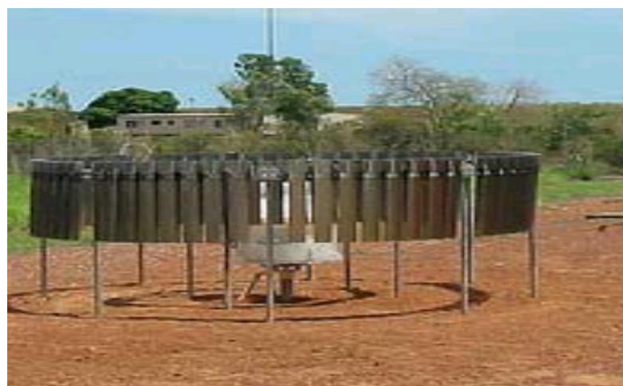
Figure 2: Weighing rain gauge (Liu, Gao, and Liu., 2013).
