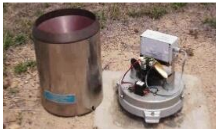
Figure 3: The tipping bucket Rain gauge (John, 2011)
