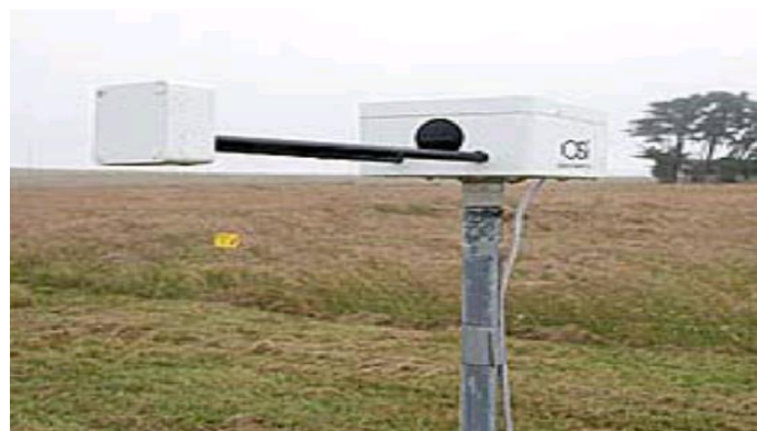
Figure 4: Optical Rain Gauge (Liu, Gao, and Liu., 2013)
