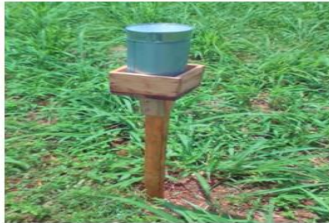
Figure 16: Assembled and mounted rain gauge for data collection
