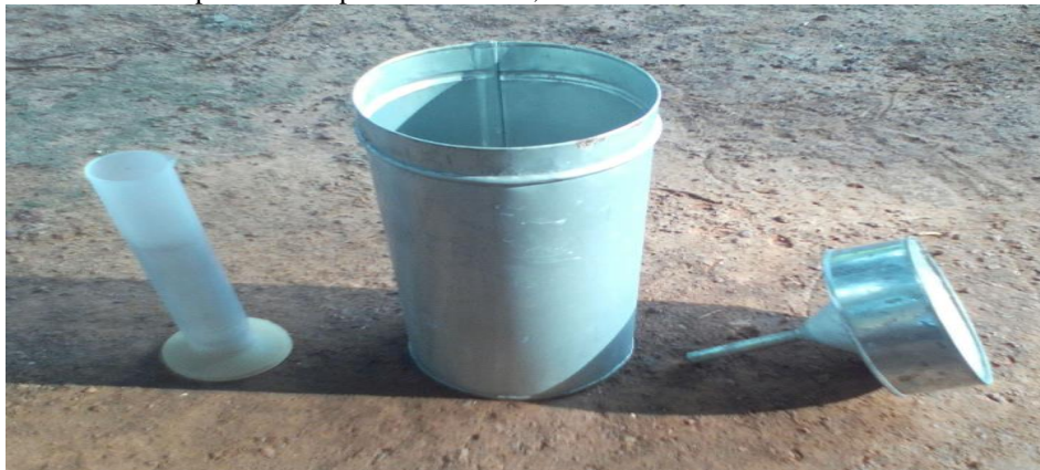
Figure 11: Three major parts of the standard rain gauge
