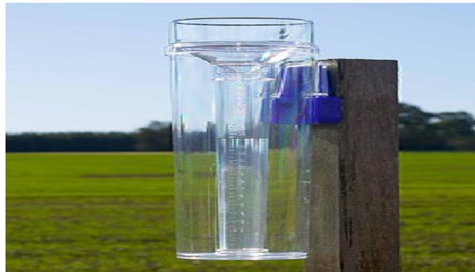
Figure 6: Standard rain gauge (Olive centre, 2012)
