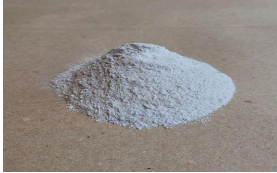
Figure 2. Lime (Stabilizing Agent)
