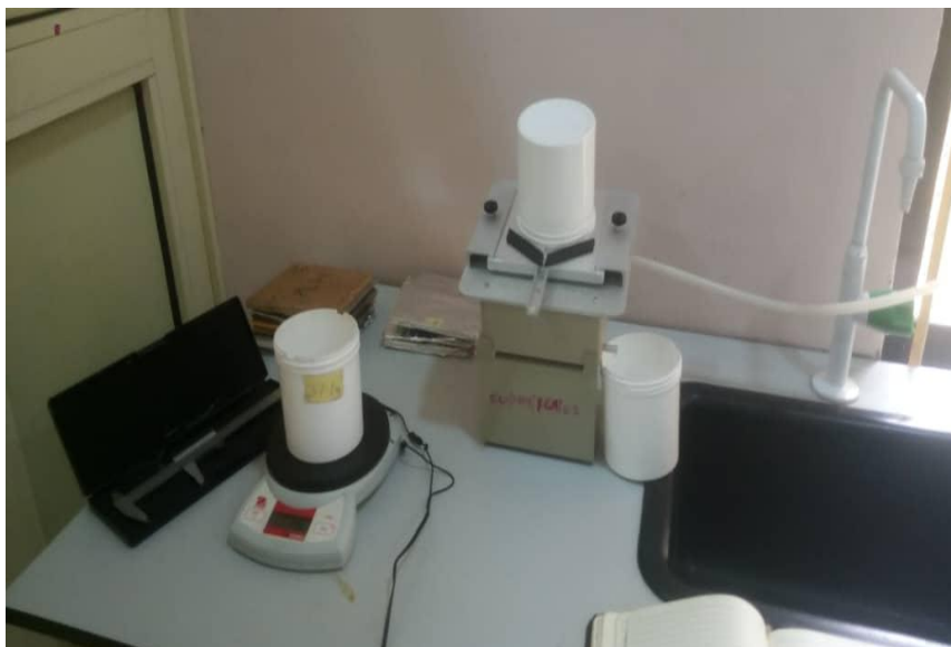
Plate 1: Laboratory thermodynamic (ice and steam) apparatus for thermal conductivity
