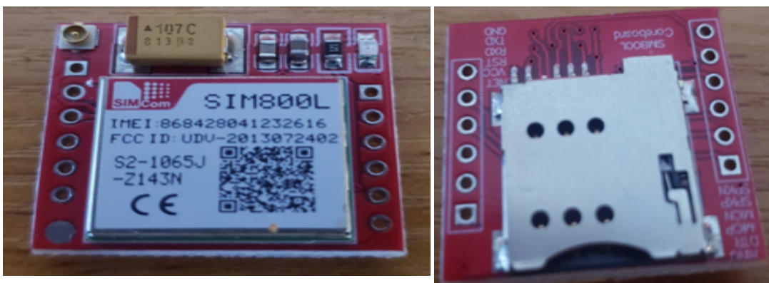
Figure 7: GSM module SIM 400 used in the design
