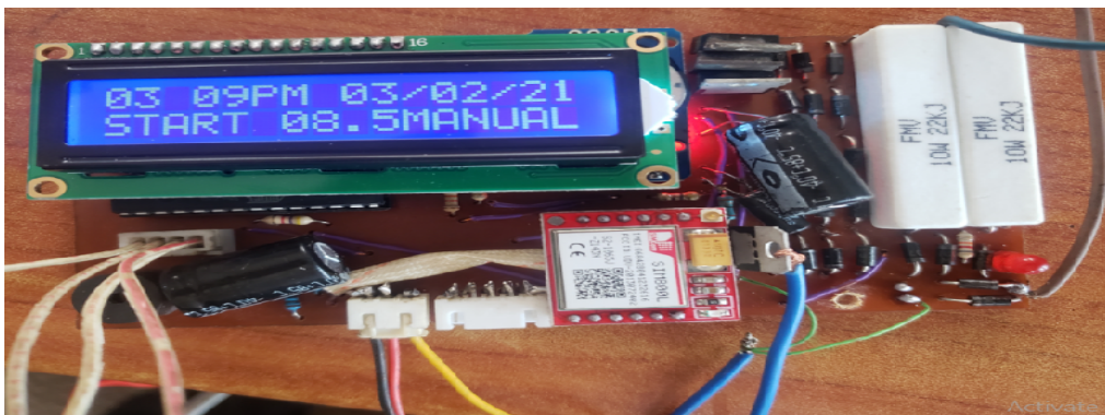
Figure 3: Soldered panel with all the components in pulse oximetry system
