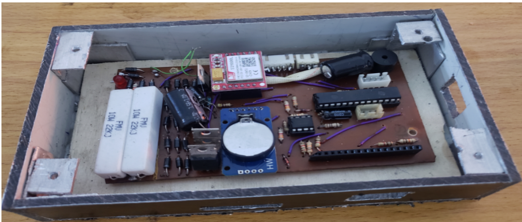
Figure 6: Fixed and tested components mounted inside the casing
