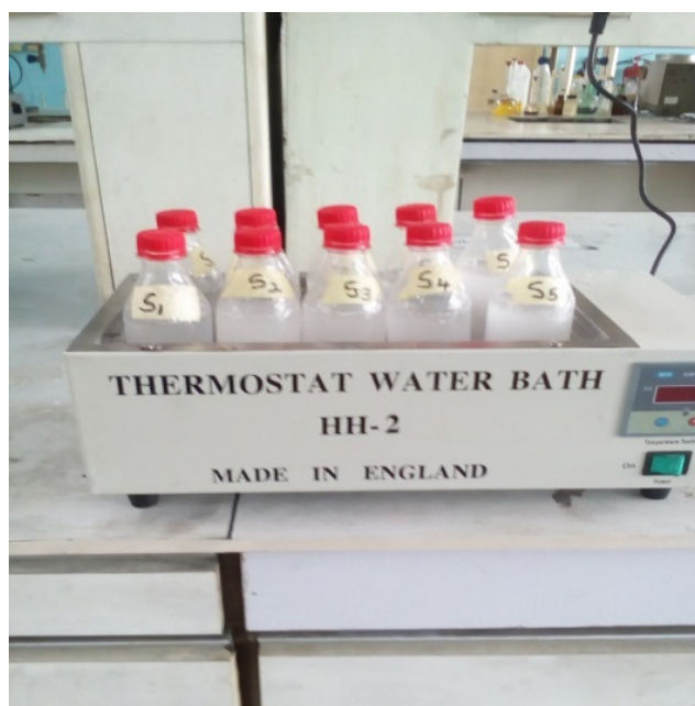
Figure 3: Experimental Set-up for Determining Cassava Wastewater (Substrate) Concentration
