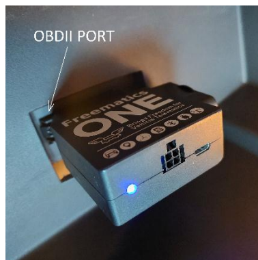
Fig. 2- Photo of the data logger used in the vehicle's OBD-II port
