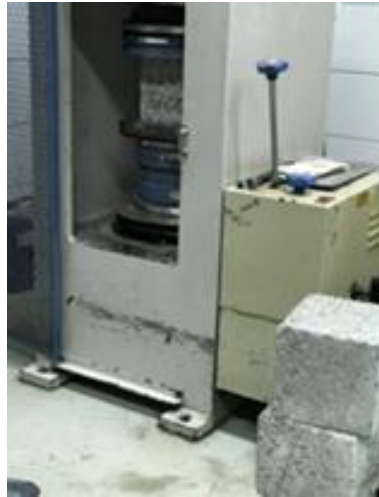
Fig. 5: Compressive strength testing machine.
