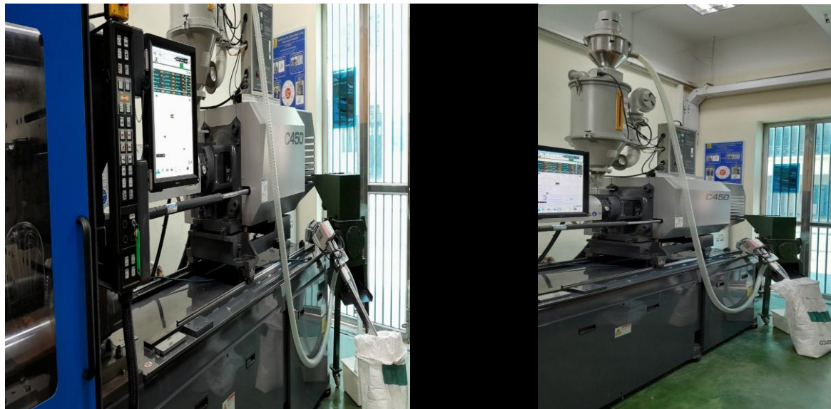
Fig. 5. The combination between the plastic granule recycling equipment and injection molding machine
