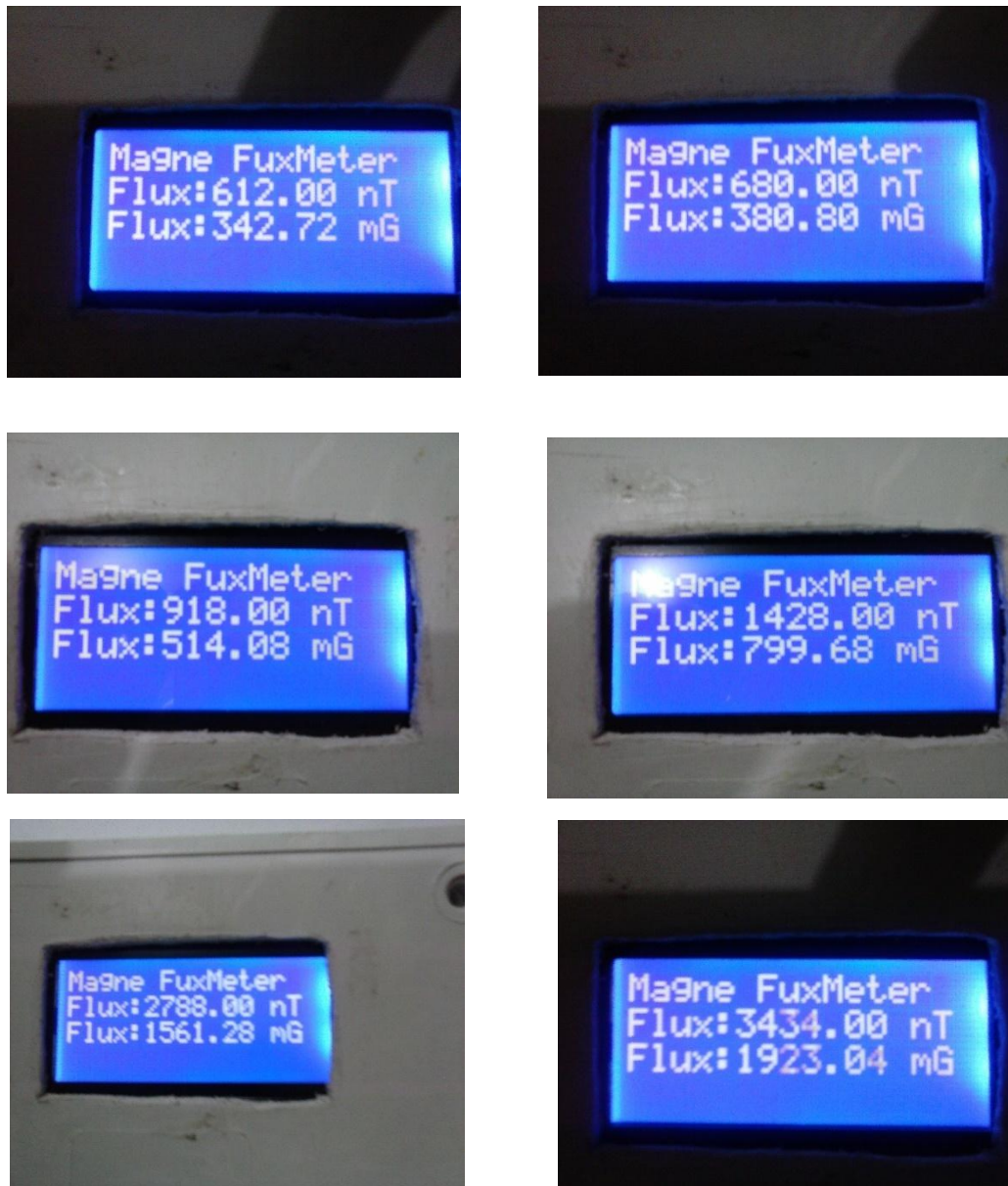
Figure 9: Showing magnetic flux readings when the developed magnetic fluxmeter is 1cm away from the Current-carrying wire at various current flows.
