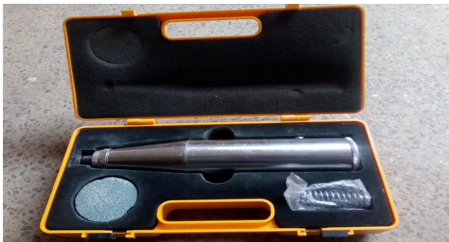
Fig. 4: Schmidt rebound hammer
