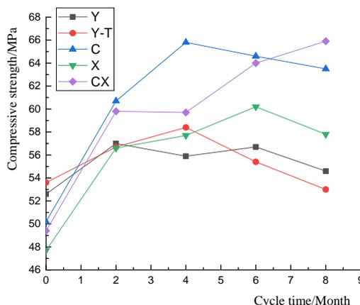
Fig.4. Time-lapse curve of concrete compressive strength
