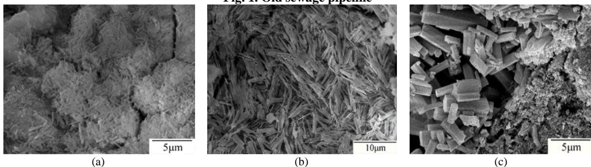
Fig.2. Microscopic morphology of concrete cement stone sample for sewage pipeline
