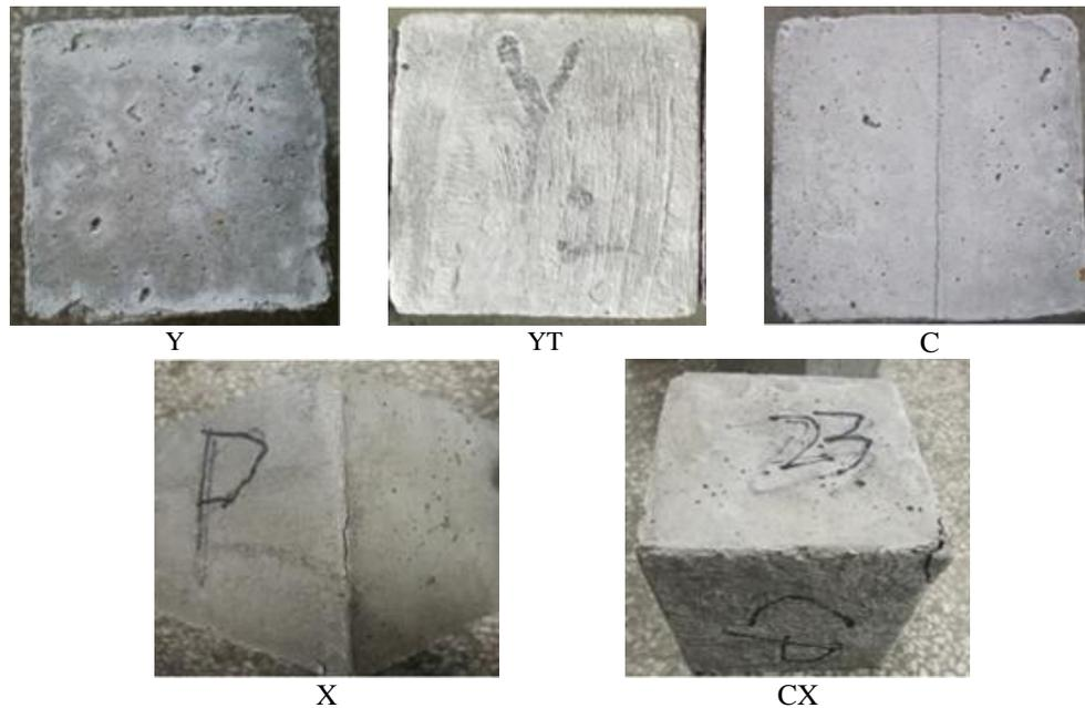
**Fig.3. Apparent quality of the test block after 8 months of dry and wet cycles**
