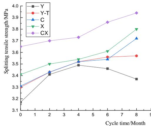
**Fig. 5. Time-dependent curve of concrete splitting tensile strength**
