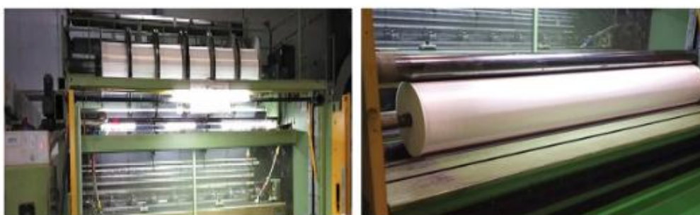
Fig. (3) Knitting of the polyester fabric
