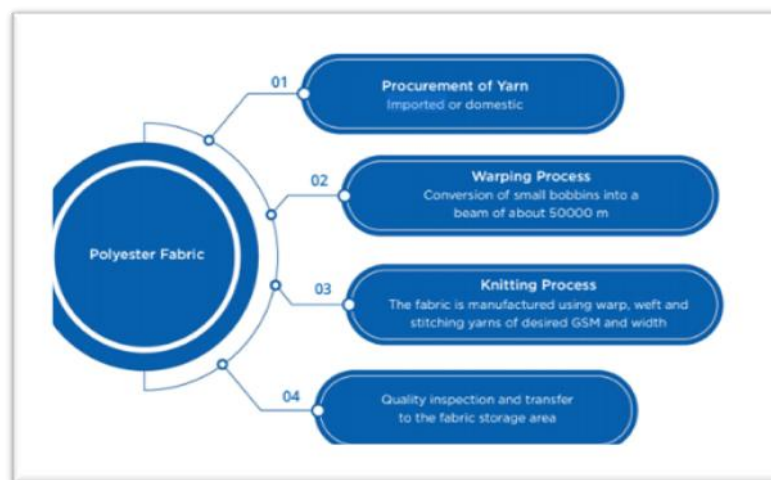
Fig. (2) Production of the polyester fabric
