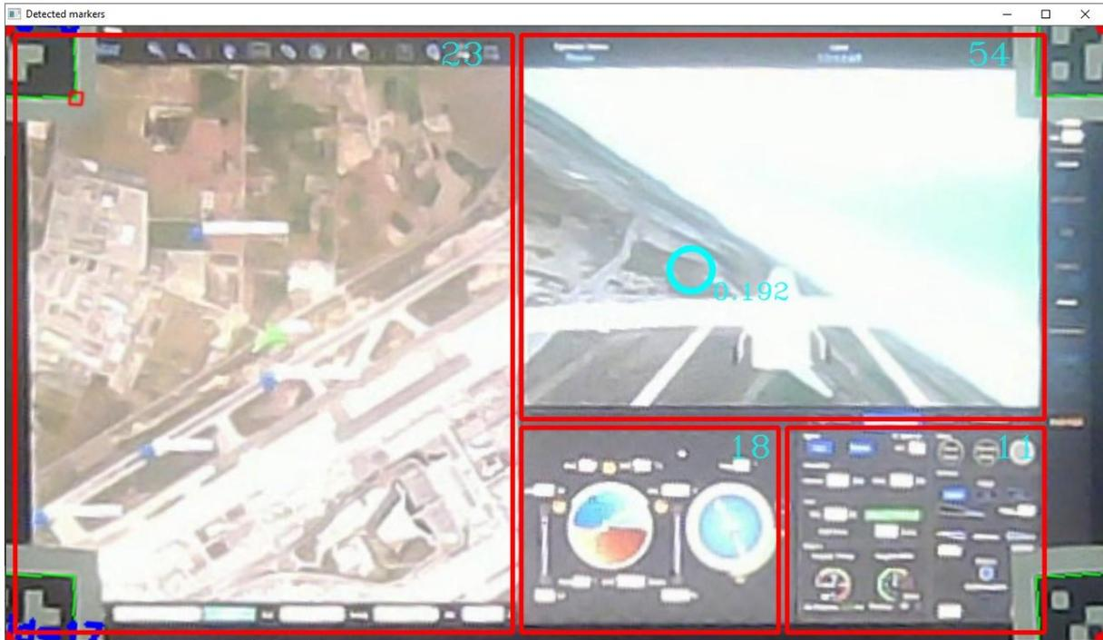
Fig. 8. Transformed region of interest with fixations being counted
