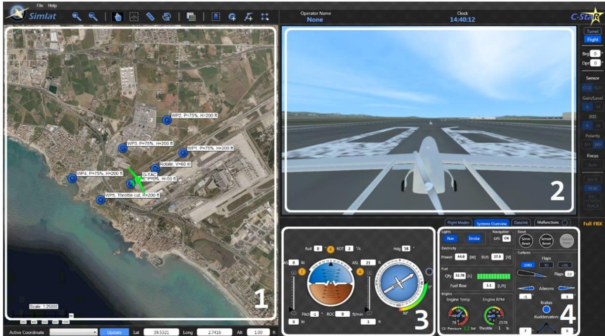
Fig. 4. Pilot station screen divided into four zones of interest
