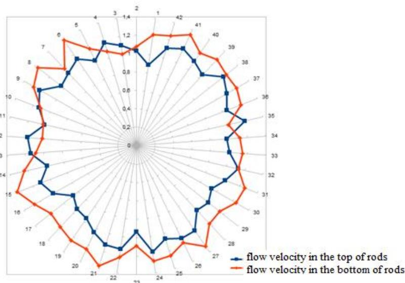
Figure 2. Diagram of the speed of water in the rods (block No. 2 of the OE KNPP).
