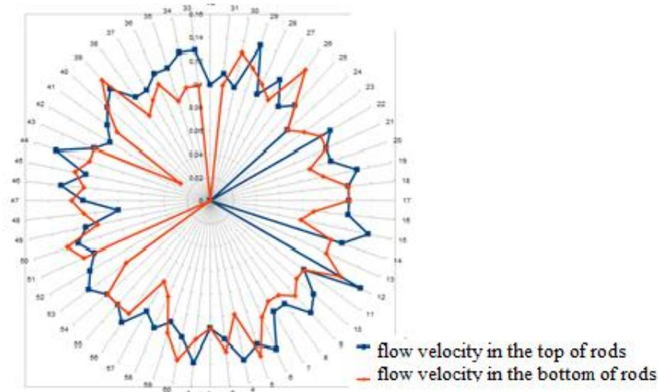
Figure 3. Diagram of the speed of water movement in the rods (block No. 1 of the OE of the SU NPP).
