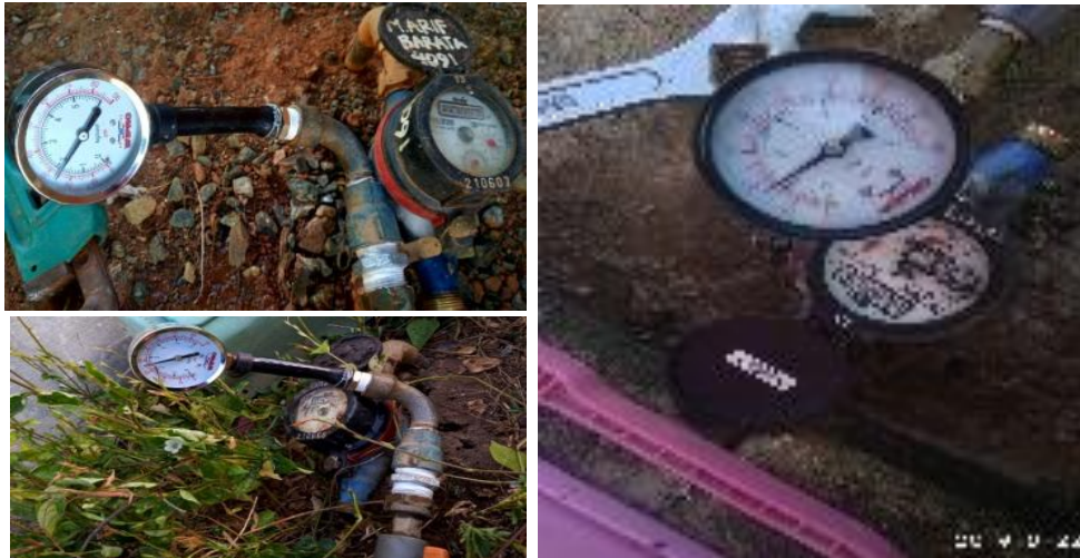
Figure 2. Calibration at several junctions
