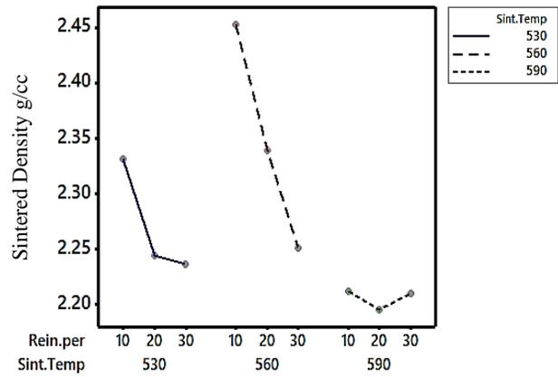
Fig.8. Individual plot for sintered density with respect to; (a) Reinforcement percentage, (b) Sintering temperature.
