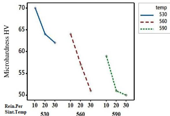
Fig.9. Individual plot for microhardness with respect to; (a) Reinforcement percentage, (b) Sintering temperature.
