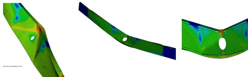
Figure 9. Finite element models failure mode results.
