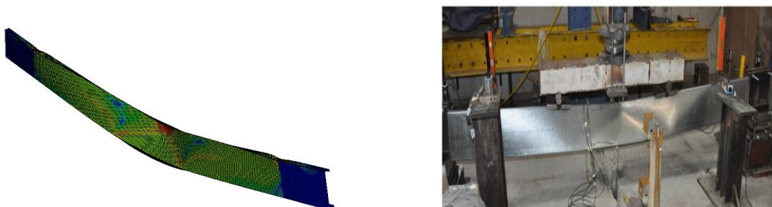
Figure 6. Comparison the FEA failure mode with the experimental results [12].
