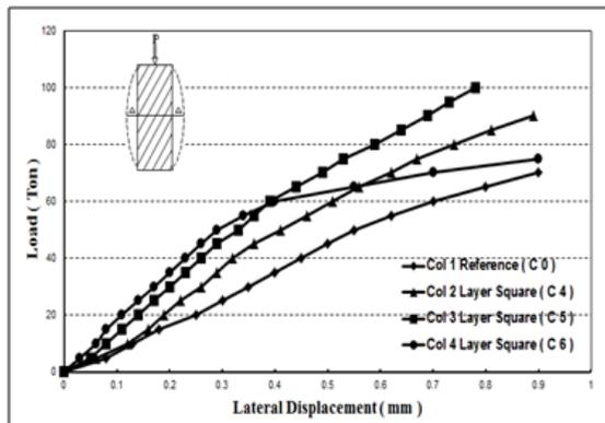
Fig. 11. Variation of load with respect to lateral displacement for columns in a group (C) compared with the reference column (A0).
