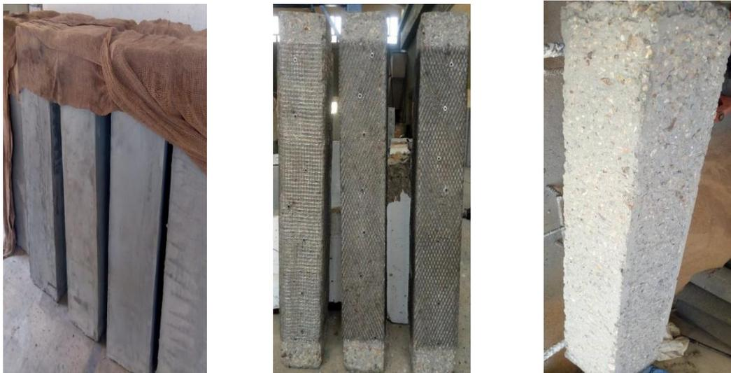
Fig. 4. Prepared of surface of columns, Jacket of columns with Ferro-cement mesh and finally casting with mortar.
