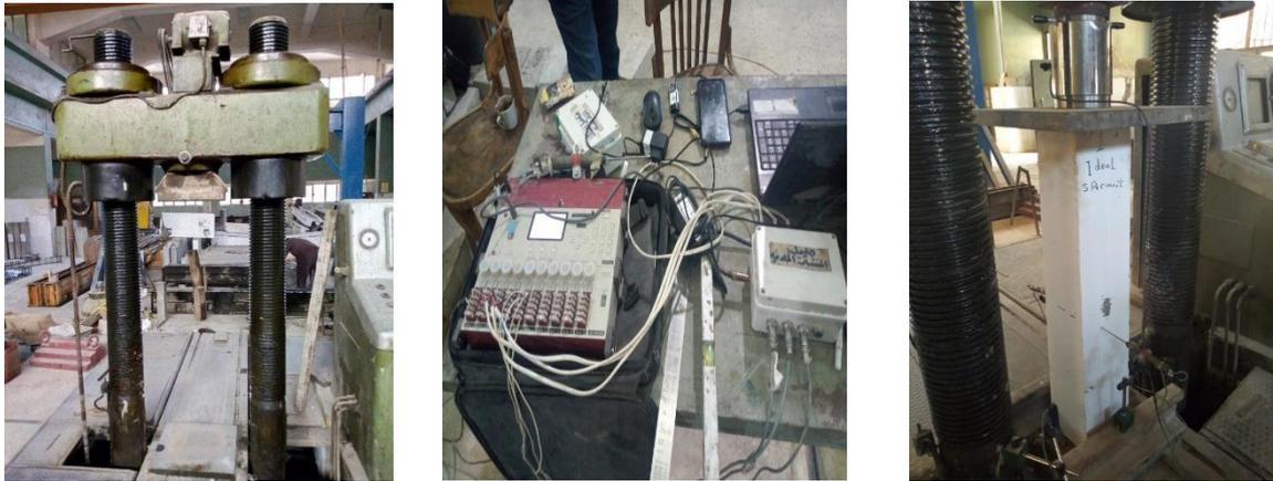
Fig. 5. Testing Machine, Data logger device and the positions of axial and lateral LVDTs on tested column
