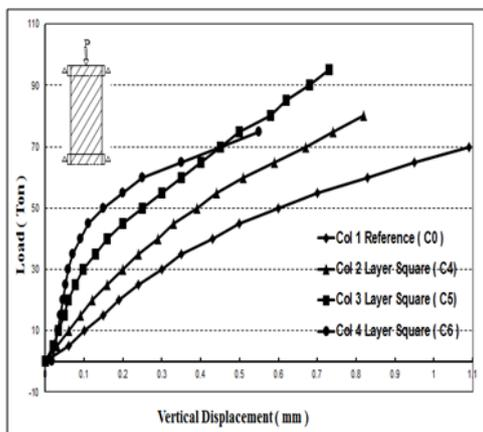
Fig. 8. Variation of load with respect to vertical displacement For columns in a group (C) compared with reference column (A0).
