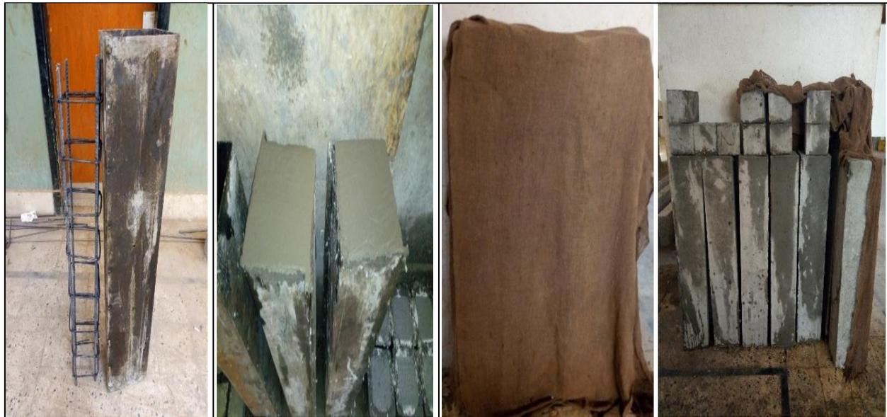
Fig. 3. Preparing of steel cage, casting and curing of the tested columns.
