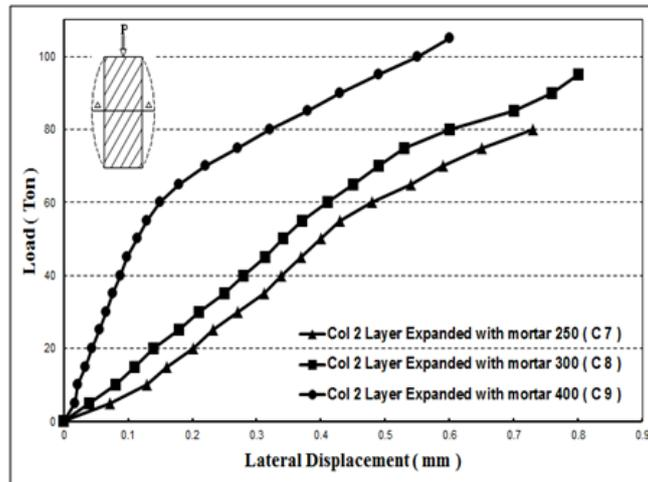
Fig. 12. Variation of load with respect to lateral displacement for columns in a group (D) compared with reference column (A0).
