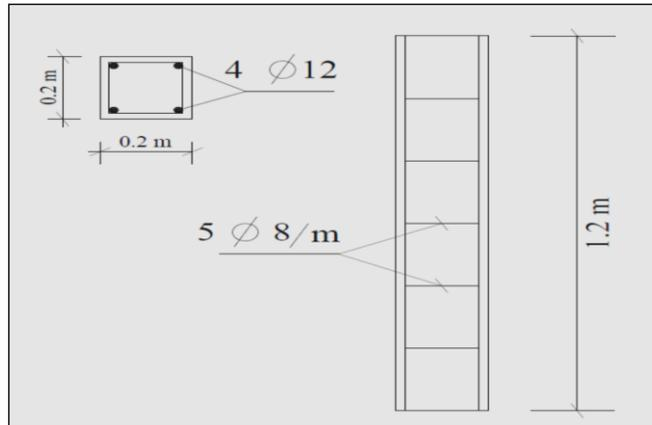
Fig. 2. Details of tested column.
