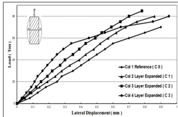
Fig. 10. Variation of load with respect to lateral displacement for columns in a group (B) compared with the reference column (A0).
