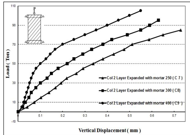
Fig. 9. Variation of load with respect to vertical Displacement for columns in a group (D).
