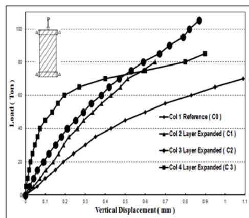
Fig. 7. Variation of load with respect to vertical displacement For columns in a group (B) compared with the reference column (A0).
